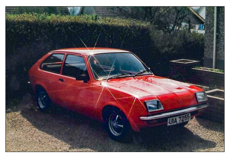
At one point in its life my Chevette developed an intermittent fault, or as I like to describe it, became possessed. The fault was almost impossible to diagnose because most of the time it was absent, but when it manifested, the symptoms were interesting. The sidelights came on with the brake lights, it wouldn't idle and indeed stalled mid gear change, and when braking and indicating the rear lights
