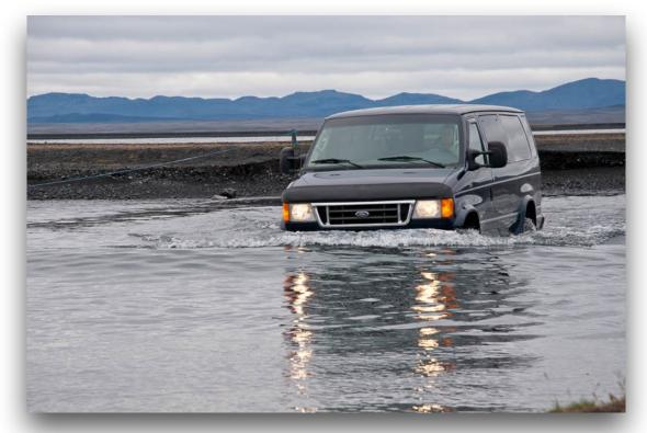
• If you are in the slightest doubt, then turn around and don't go through the flood. Often modern saloon cars have the air intake in the wheel arch, which may be below the water level. If your engine should take in water, it will immediately hydro lock and the engine will stop.
