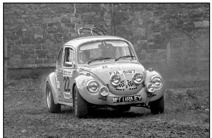
Ulster Rally 1976 (note the oil cooler mounted on the roof)
